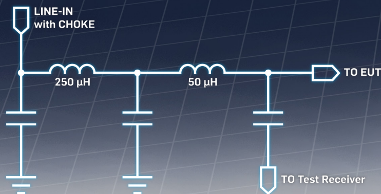
L3-32 equivalent circuit
