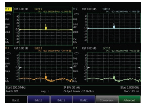
Characterized common and differential mode reflections with mixed-mode S-parameter measurements
