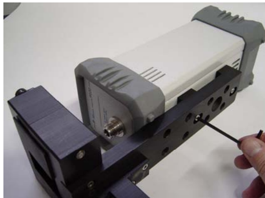
Fig. 11-13 Mounting the Antenna Holder on PMM 9030/9060/9180
