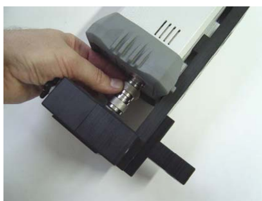
Fig. 11-14 Screwing the N-N Adapter for Antenna Matching
