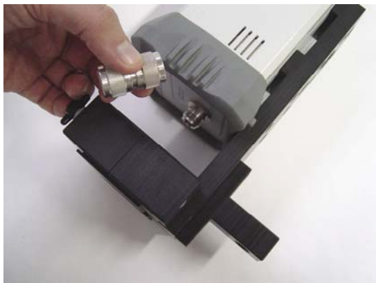
Fig. 11-14 Screwing the N-N Adapter for Antenna Matching
