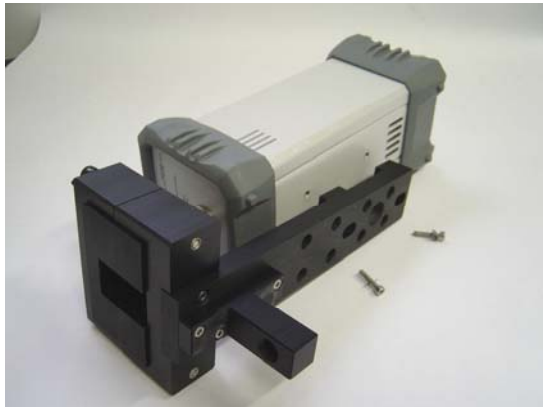
Fig. 11-13 Mounting the Antenna Holder on PMM 9030/9060/9180
