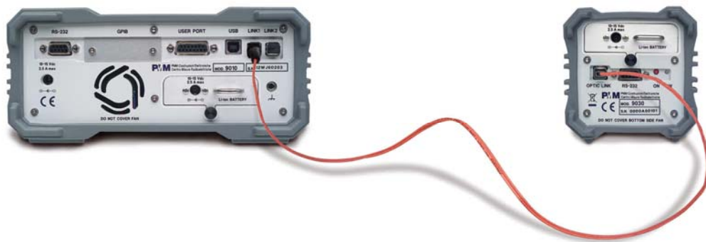
Fig. 11-5 PMM 9030/9060/9180 Fiber Optic Link to PMM 9010
