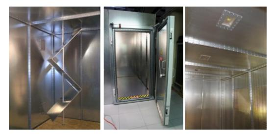
Electromagnetic reverberation chamber is a multifunctional **EMC** (Electromagnetic Compatibility) test facility for commercial, military, automotive testing and other electromagnetic investigations. Also known as <u>reverb chamber</u> (**RVC**) or <u>mode-stirred chamber</u> (**MSC**) or, <u>Vibrating intrisic reverberation</u> <u>chamber</u> (**VRC**).
