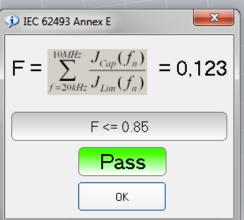
IEC 62493 requires the exposure of humans to the EMF generated by lighting devices to be assessed by measuring the RF field with a special sensor - the Van der
