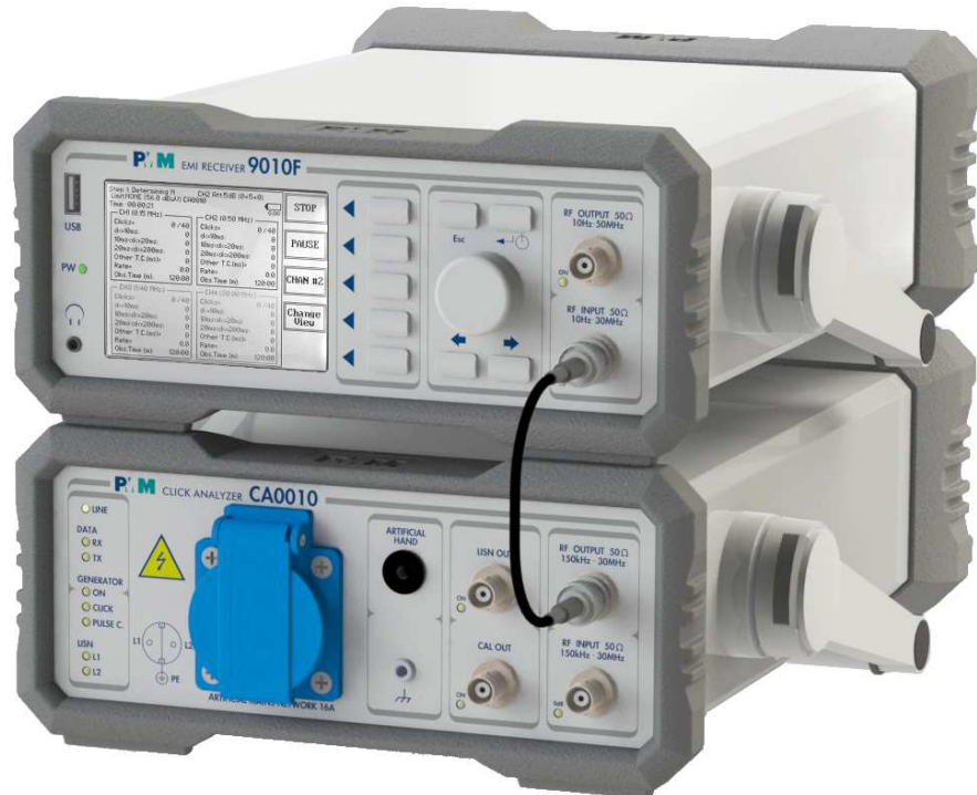
Fig. 2-1 PMM CA0010 click analysis setup.
