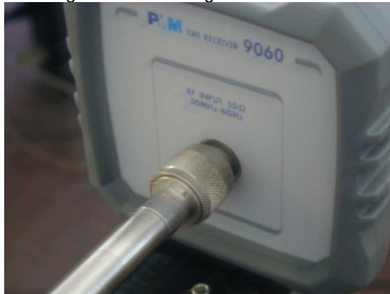
Attaching PMM LP-03 Log Periodic
