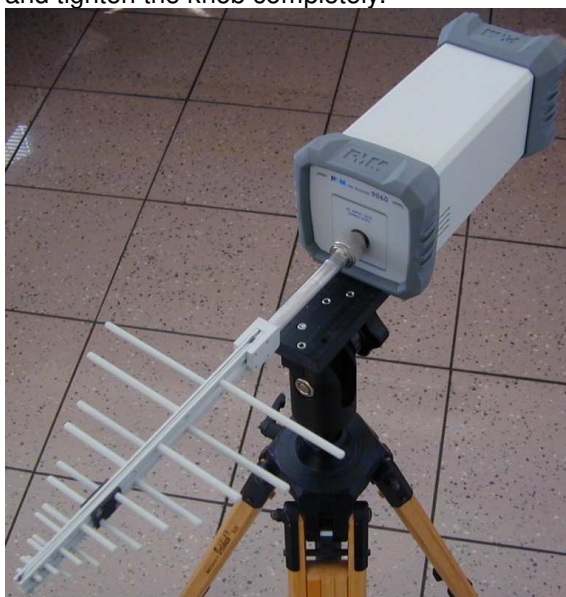
Change the PMM 9060 polarization from horizontal to vertical or vice versa and tighten the knob completely.
