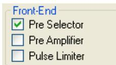
To provide proper investigation tools in Analyzer and Manual Modes some additional tick boxes are provided for enabling/disabling internal **Front End** devices.
