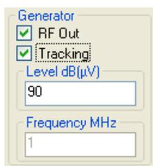
PMM 9010 and PMM 9010/30P receivers are equipped with an embedded RF Generator which can be activated for some checks about RF Input features or about cables' losses and band-pass behaviour of external filters and attenuators.
