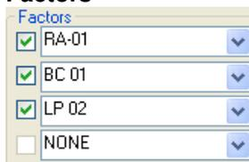
When you use one or more devices added externally to the receiver (Antennas, LISNs, Cable, Attenuator, Amplifier, near field probes, etc), you may take proper account of losses; in the Factors box you can load the correction factors defined in the Factor tool (see General functions chapter). In this way the Software will correct the absolute measurement adding or subtracting the correction factors frequency by frequency.
