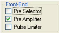
The **Pre-Amplifier** selection is available in every Operation Mode, but in particular for the Sweep Mode it has been included in the Table settings below the Graph screen, to be more flexibly selected in each row according to each specific frequency slice.
