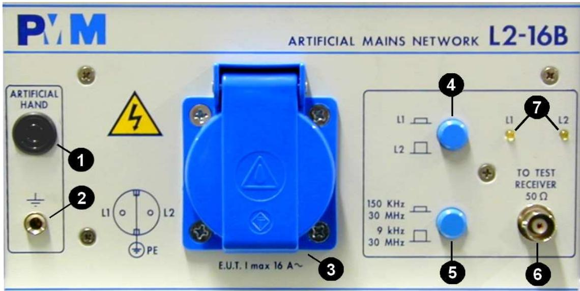
**Fig. 3-5** Front Panel
