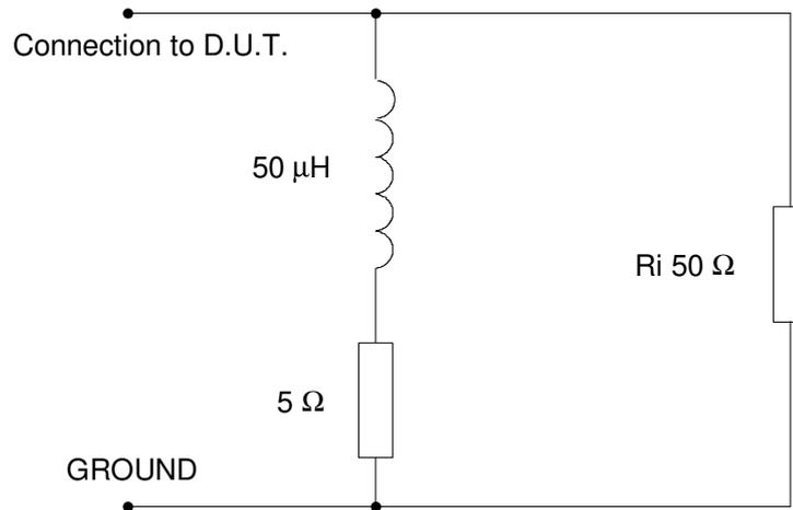
$R_i$  = input impedance of the RFI
