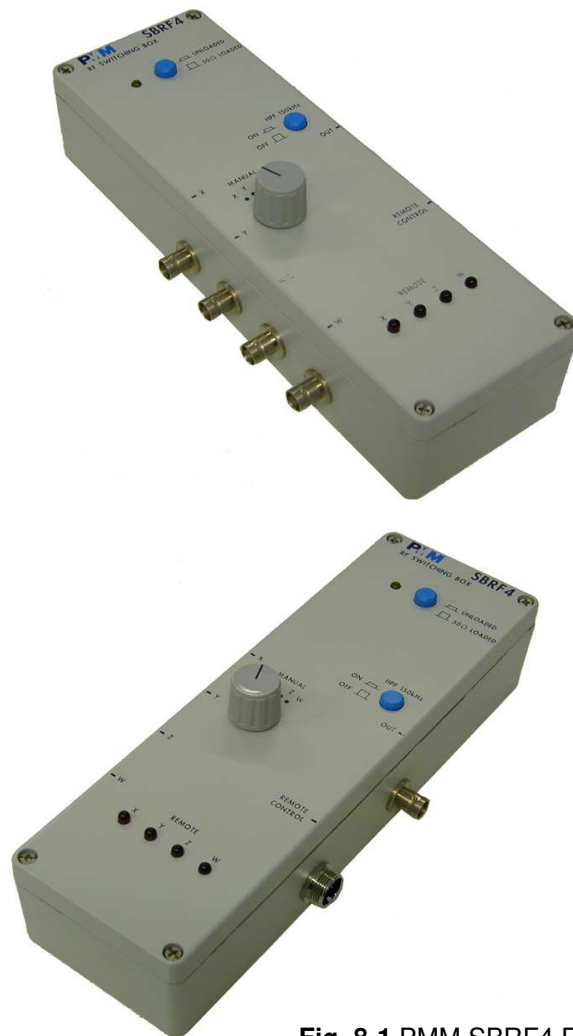
Fig. 8-1 PMM SBRF4 RF Switching Box
