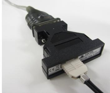
In case of 40m Fiber Optic Optional Cable **FO-EP600/40**, differently from what available for the 10m and 20m fiber, the “white plug” is not provided on one side of the fiber for 8053-OC Adapter matching.
