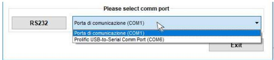
When the USB connection is used, the USB-RS232 adapter appears among the devices as a “Prolific USB to Serial Comm Port (COMn)”.
