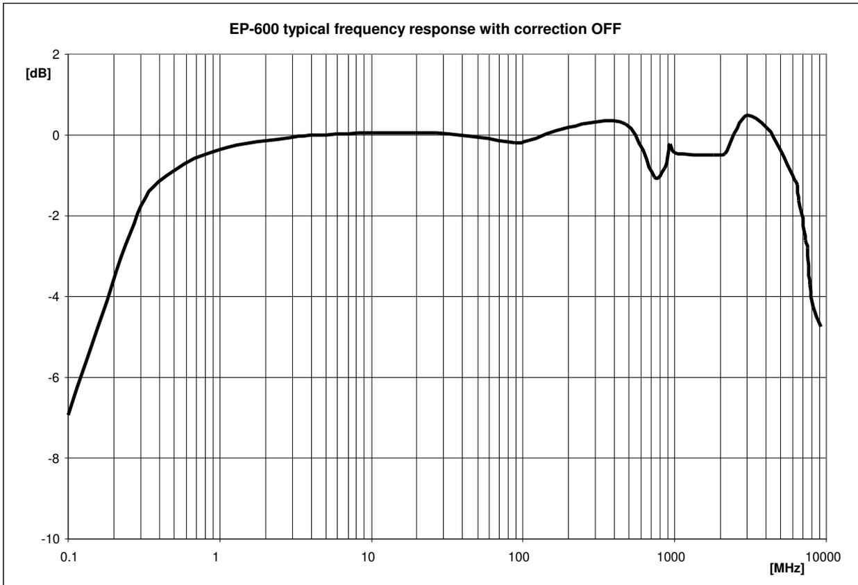
**Fig. 1-3** EP-600 typical frequency response with correction OFF
