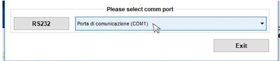
When the menu is selected, the communication port selector appears. It allows the user to choose between the RS232 port or RS232-to-USB converter that is needed if no RS232 port is available in the controller PC.
