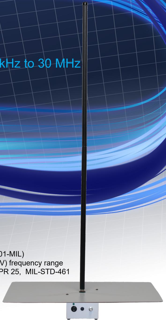
RA-01 Rod Antenna is an active monopole antenna built to CISPR 16-1-4 specifications and perfect for RF electric field measurements in a wide variety of EMC applications. The RA-01-HV model is ruggedized to be able to withstand 50 Hz electric fields as high as 8 kV/m, and is therefore best suited to performing interference measurements in close proximity to high-voltage power lines.
