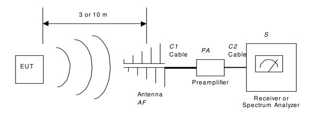
Fig. 3-1 Radiated emission test setup
