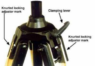
Fig. 1-29 Adjustable joint
