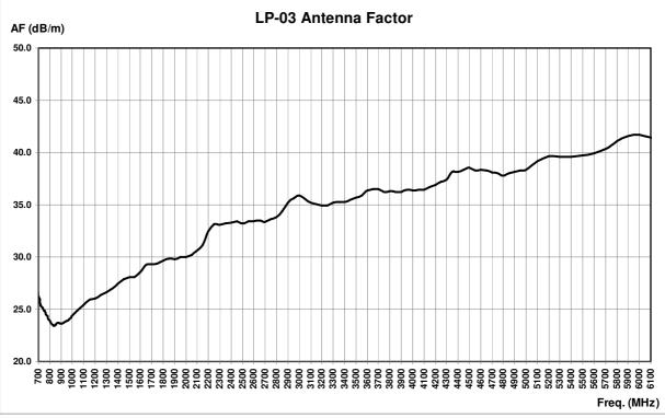
Fig. 1-21 Typical LP-03 antenna factor
