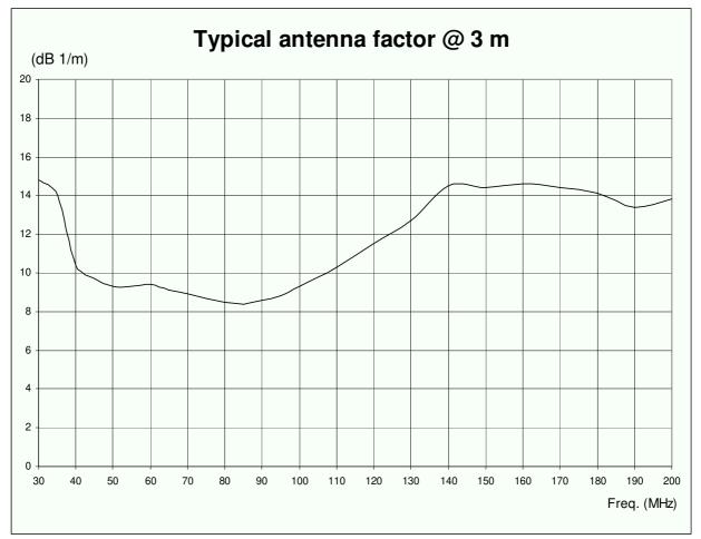
Fig. 1-14 Typical BC-01 antenna factor @ 3 m
