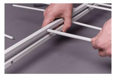
Assembly the 366mm length cylindrical dipole to the boom
