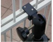
Change the antenna polarization from horizontal to vertical or vice versa and tighten the knob completely.
