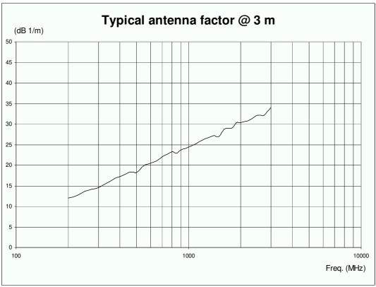
Fig. 1-18 Typical LP-02 antenna factor @ 3 m
