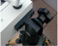
Change the antenna polarization from horizontal to vertical or vice versa and tighten the knob completely.
