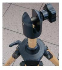
Remove the screws from the tripod joint.
