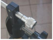
Change the antenna polarization from horizontal to vertical or vice versa and tighten the knob completely.
