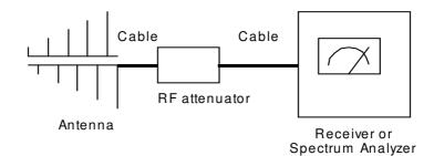
Fig. 3-3 Environmental test setup
