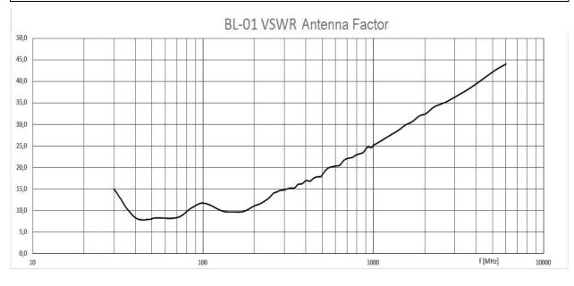
Fig. 1-16 Typical BL-01 antenna factor
