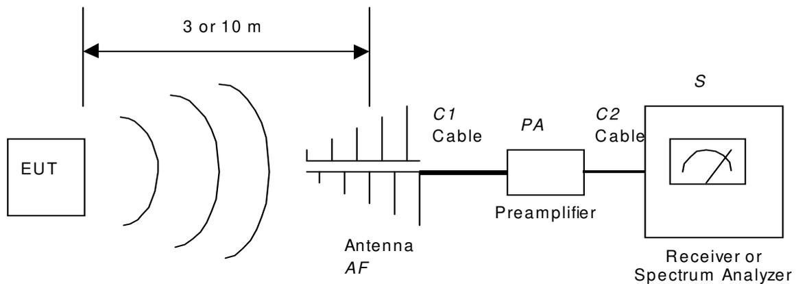
**Fig. 3-1** Radiated emission test setup
