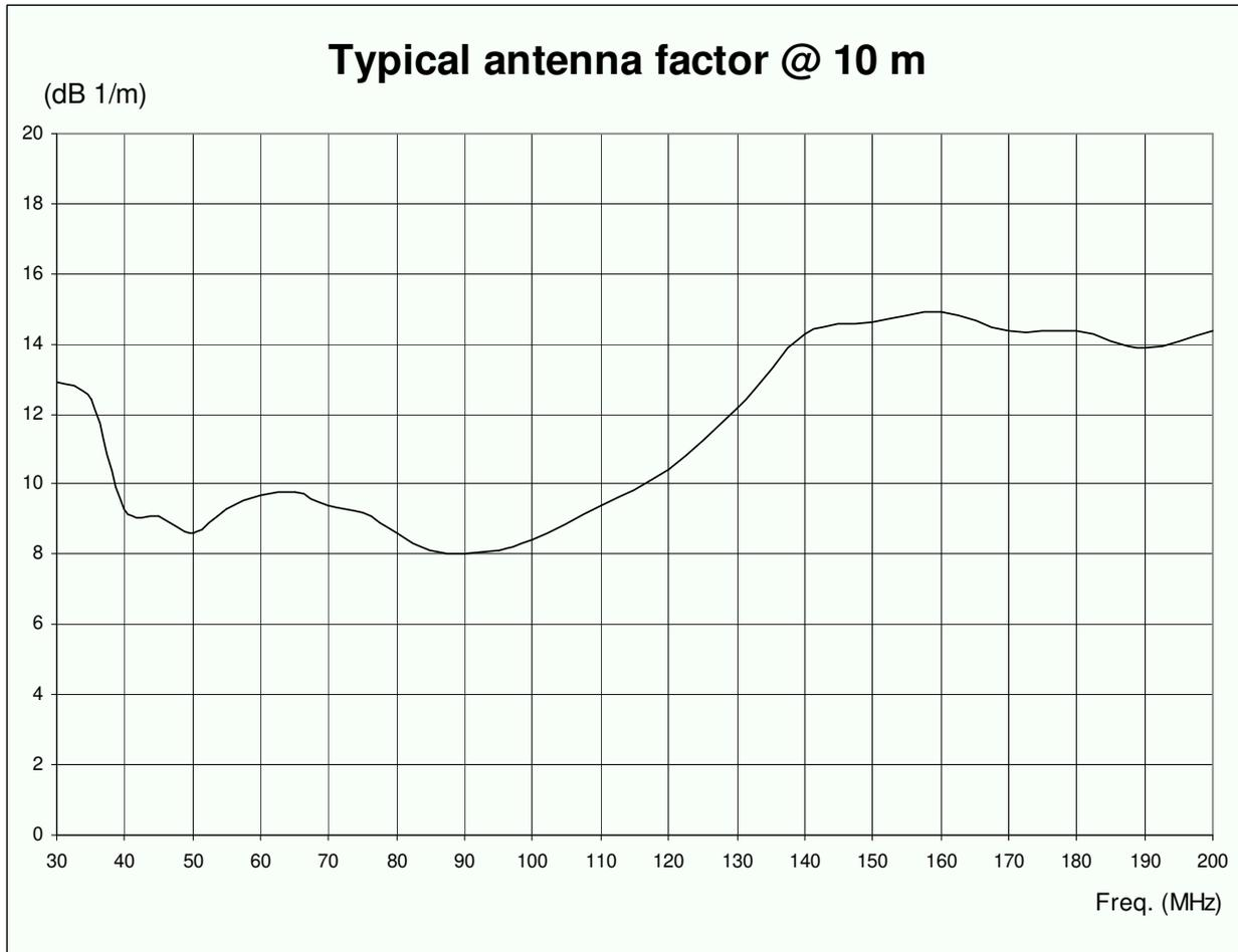
**Fig. 1-15** Typical BC-01 antenna factor @ 10 m
