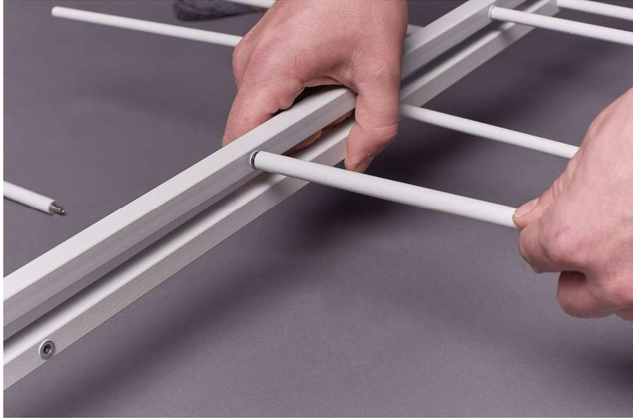
Screw the two longer cylindrical dipole (449.5mm length) to the boom
