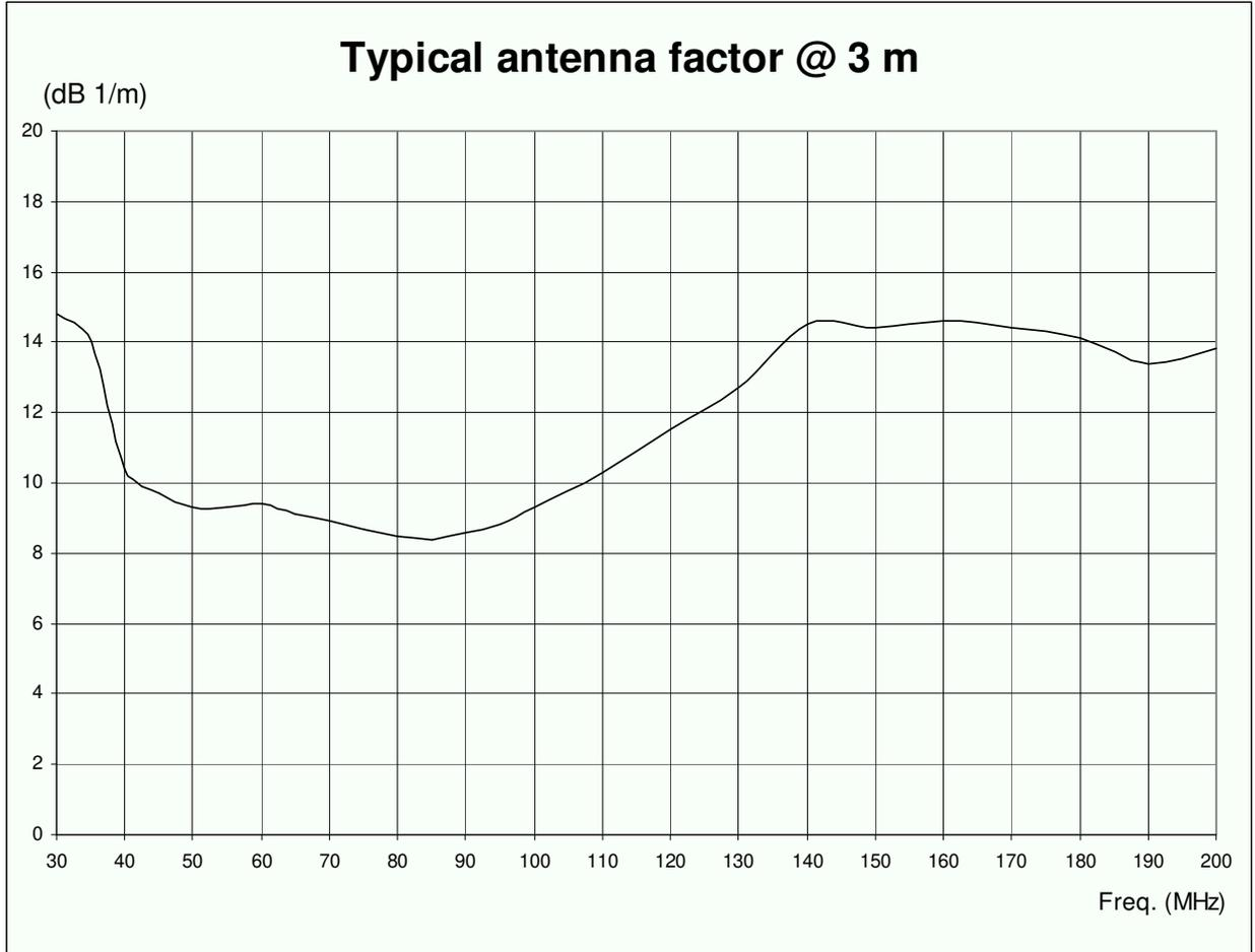
**Fig. 1-14** Typical BC-01 antenna factor @ 3 m
