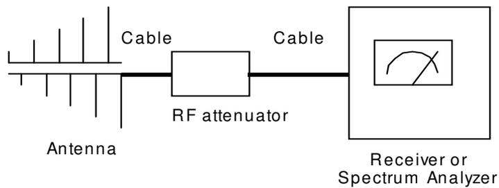
**Fig. 3-3** Environmental test setup
