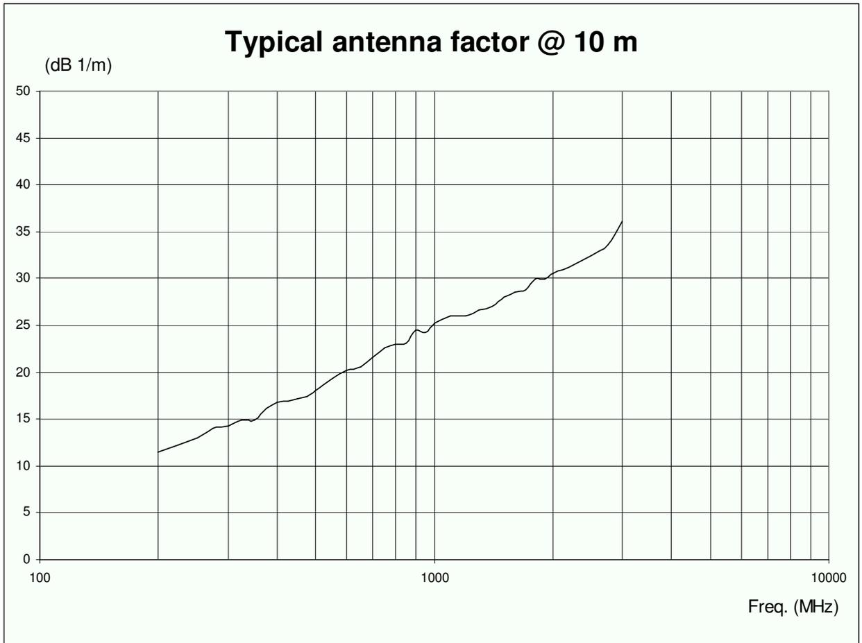
**Fig. 1-19** Typical LP-02 antenna factor @ 10 m
