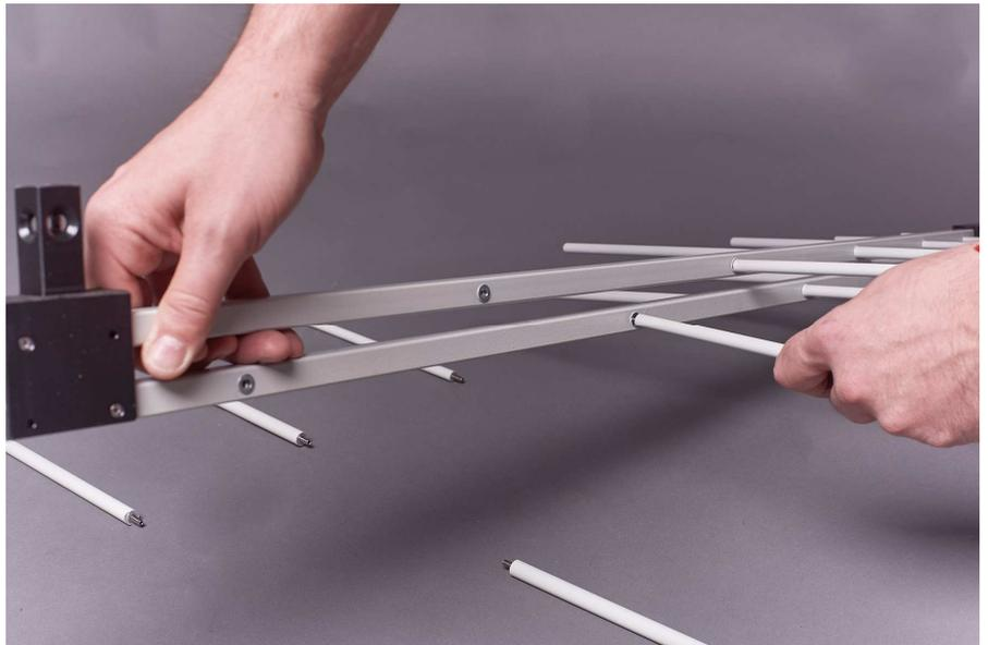
Assembly the 366mm length cylindrical dipole to the boom
