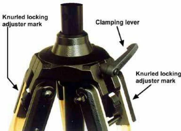
**Fig. 1-29** Adjustable joint
