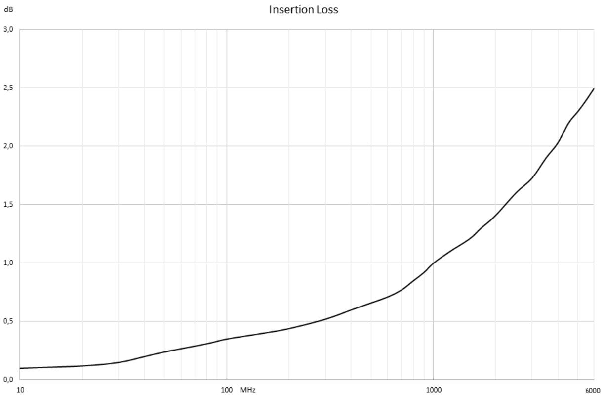
**Fig. 1-30** Typical RF Cable/5 insertion loss
