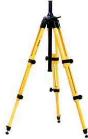
**Fig. 1-28** Mounting head with center column
